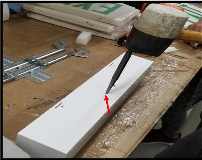
Using a Philips screwdriver or some other sharp tool, punch out the knockouts creating holes
