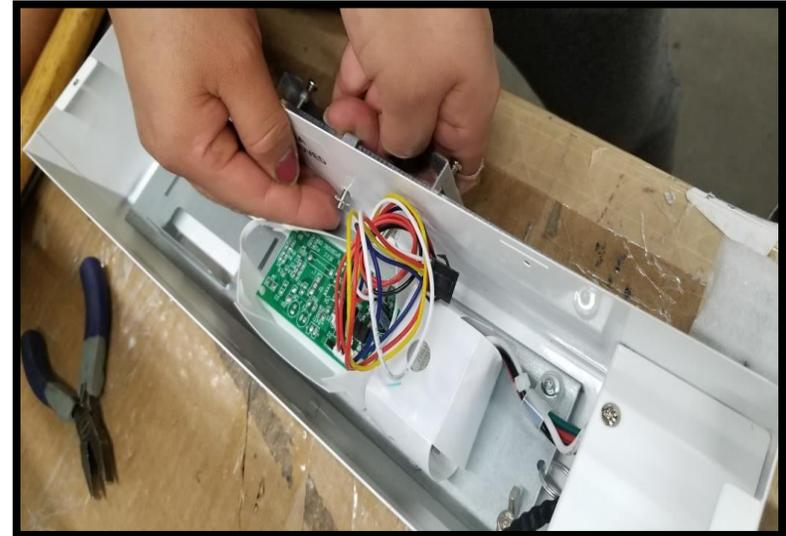
Using the screws and wingnuts secure the bar hanger to the housing
